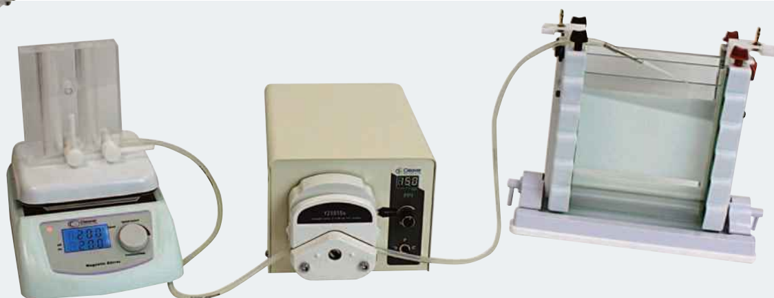
Casting process for DGGE gels
