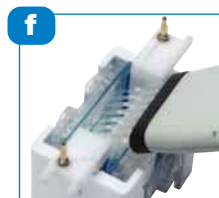
Load samples using Loading Guides and run
