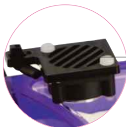
USB powered extraction fan
