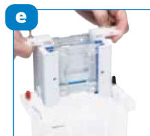
Transfer to tank and fill with buffer
