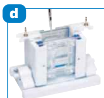
Insert gel solution and comb and allow to polymerise
