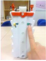
3. Push the green sliding gel clamp out of the PAGE insert by gently pressing the protruding pin as shown.
