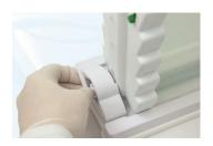
6. With the cam pin handles facing directly downwards, turn the cam pins fully through 135° or until the insert has tightened onto the silicone mat.
