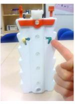
To replace the green sliding gel clamps, begin by unscrewing the colour-coded vertical screw pins. There should be no glass plates within the PAGE insert, in the side(s) being unscrewed. Once the screw pins are unscrewed sufficiently the green clamp should sit in the resting slot as shown.
