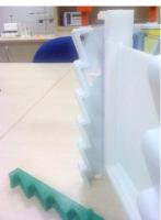
4. Once the green sliding gel clamp is removed the PAGE insert is ready to accept the thinner yellow sliding gel clamps for 2-gel sandwiches, either side of the PAGE insert, to convert the WAVE to a 4-gel configuration.
