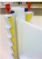
6. Withdraw the sliding gel clamps so that they sit suspended in the resting slots as shown. Repeat steps 1-6 to replace the remaining green sliding gel clamps. Once complete the PAGE insert is ready for 4-gel assembly.
