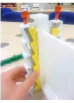
5. Insert the yellow sliding gel clamp into the hole closest to the core of the PAGE insert. Once inserted gently withdraw the sliding clamp outwards away from the core of the PAGE insert as shown.
